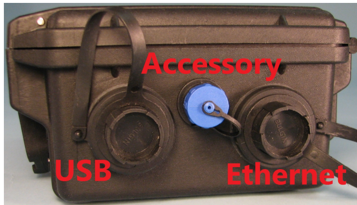
Figure 22: Topside Communications Unit (TCU) Right View
