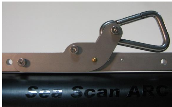
Figure 45: Reinstall the Tow Fish Safety Release
