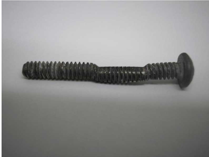
Figure 34: Worn Shear Pin in Need of Replacement
