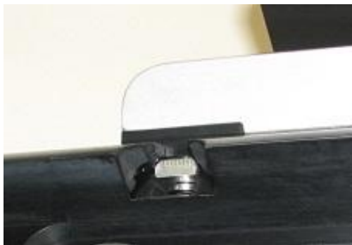
Figure 41: Tow Rail Nut Aligned with the Tow Fish Angle Adjustment Groove
