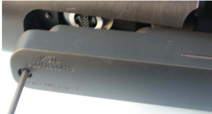
Figure 30: Screw removal to access a transducer
