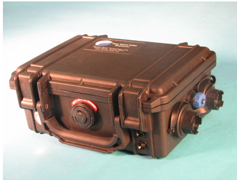
Figure 16: Topside Communications Unit
